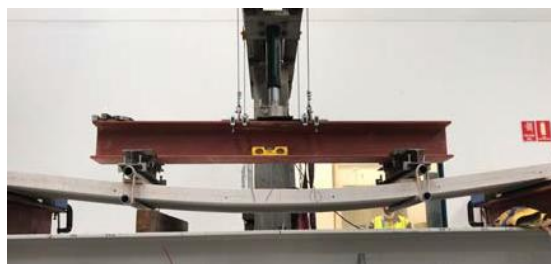
Figure 5 - Structural testing of 75mm E-METRIX®
