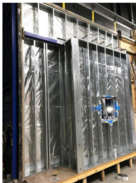
Figure 6 - Weatherproofing testing of 75mm E-METRIX®
