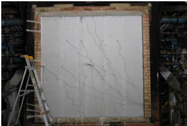
Figure 7 - Fire testing of 75mm E-METRIX®
